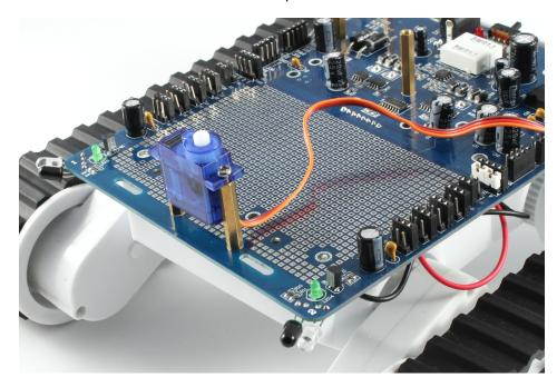
6. Put the motor wires and the battery holder into the Rover 5 chassis, and use then the long self tapping screws to attach the Explorer PCB to the Rover 5 chassis. **Tip:** It can be tough to cram all of the wires into the base, a bit of blu-tak and/or sellotape can be very useful here to hold wires in place.
