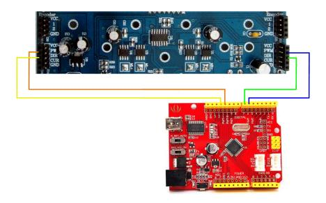
11. Wire up the encoders. The connections to make are Digital 2 to Right Encoder 1, Digital 4 to Right Encoder 2, Digital 3 to Left Encoder 1, Digital 5 to Left Encoder 2.
