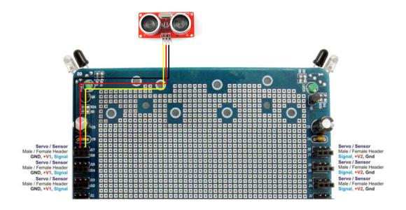
20. Now connect signal wires for the pan/tilt servo motors, and for the ultrasonic sensor to the Seeeduino. The connections to make are Digital 8 to J16 Signal, Digital 9 to J14 Signal, and Digital 10 to J12 Signal.
