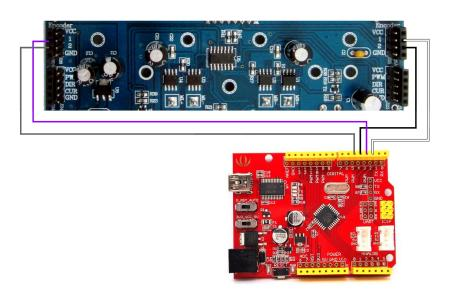
12. Use the supplied jumpers to connect IR LEDs 1 and 2, and IR LEDs 3 and 4 together.
