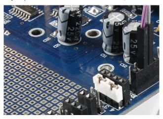
13. Wire up the corner mounted IR LEDs. The connections to make are Analog 0 to Signal In 1, and Analog 1 to Signal In 3.
