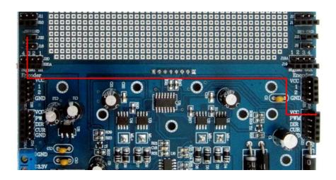
18. Connect the servos for the pan/tilt neck to the Explorer PCB. The servo wires are coloured as follows; Ground is **brown**, VCC is **red** (and in the centre), and the Signal wire is **orange**. The connections to make for the pan servo are Ground to J15 GND, VCC to J15 +V1, and Signal to J15 Signal. The connections to make for the tilt servo are Ground to J13 GND, VCC to J13 +V1, and Signal to J13 Signal.
