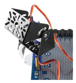
16. Use the sensor fixing set to attach the ultrasonic sensor to the pan/tilt head
