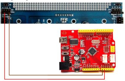
14. Wire up the corner mounted IR sensors. The connections to make are Analog 2 to Signal Out 1, Analog 3 to Signal Out 2, Analog 4 to Signal Out 3, and Analog 5 to Signal Out 4.
