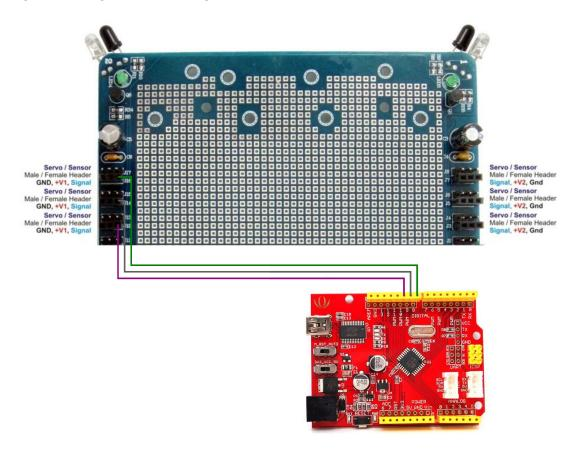
21. Wire up the motor current sensors to the Seeeduino. This will let the Seeeduino sense when a motor has stalled. The connections to make are ADC6 to left CUR and ADC7 to right CUR.
