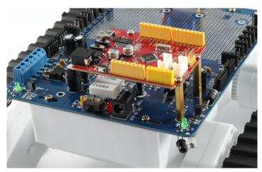
8. Connect power to Seeeduino using 2 wires (Brown and Red are good) from the set of 40 male to male jumper wires, as shown on the diagram below. Things can be kept tidy by wrapping excess wire length around the brass standoffs. The connections to make are VCC to 5V and GND to GND. **Note:** Ensure that the Seeeduino voltage is set to 5V.
