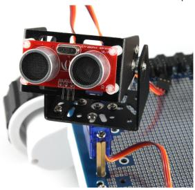
17. Now connect 5V power to the left hand power line. The connection to make is VCC to J22 SRV.
